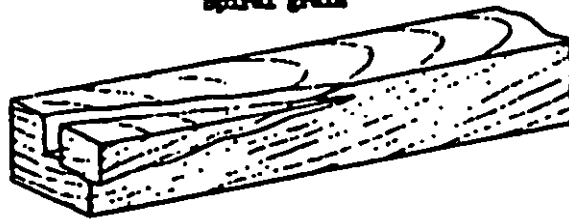
Spiral and diagonal grain in combination
